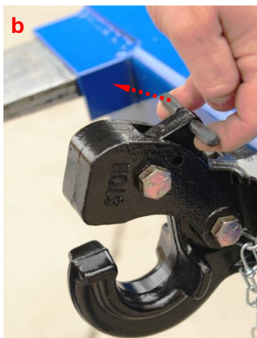
Press upwards on upper jaw and press opening lever forward
