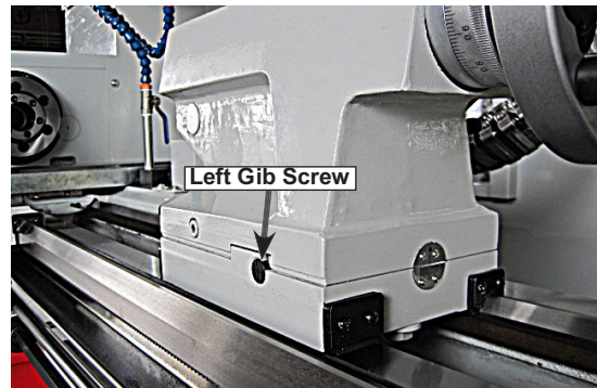
Figure 86. One of two tailstock gib screws.
