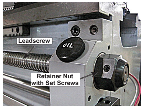
Figure 82. Leadscrew end play adjustment.
