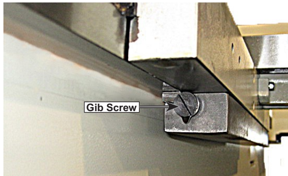
Figure 84. One of two rear saddle gib screws.
