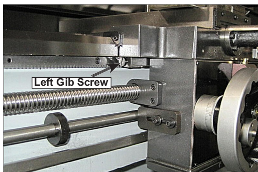
Figure 85. One of two front saddle gib screws.
