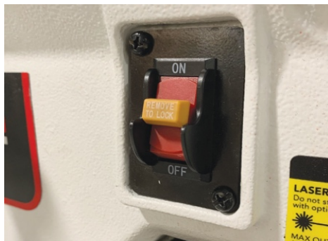
Figure 4-1: Main Power Switch
