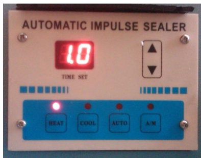
Figure 2. KS-FS Timer Control Panel
