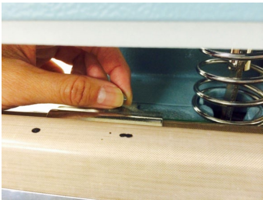
Figure 7. Screw element in place
