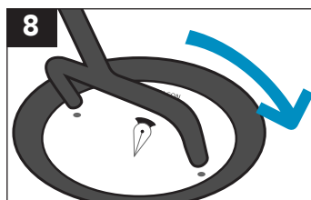
Insert new cartridge into housing and turn key to right to lock and click into place.
