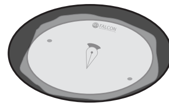
Fluid does not drain into the cartridge
