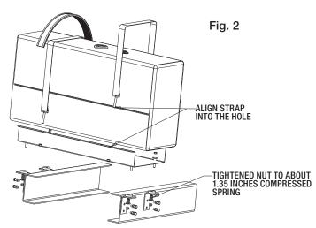
**8.** Tightened the spring bolt until the rubber conformed to the tank bottom. The spring must be compressed to about 1.35 inch. Do NOT over-tightened the spring to fully compressed.
