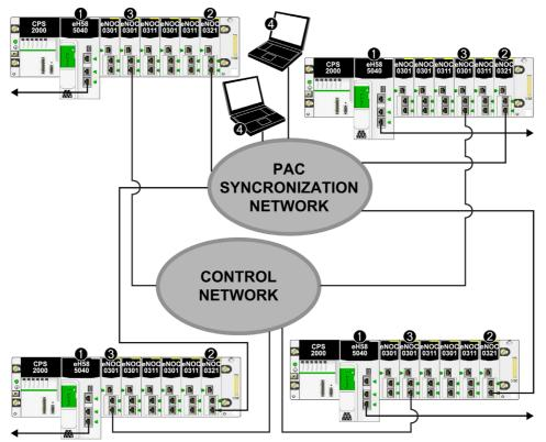
1 BMEP585040 CPU with Eternet I/O scanner service connecting to the device network
