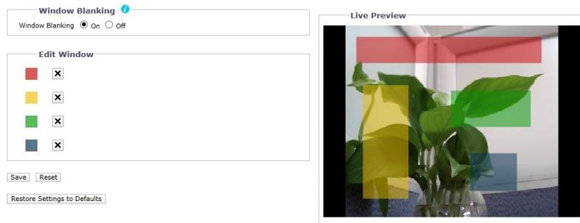
FIGURE 3-27: WINDOW BLANKING ON
