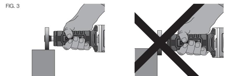
**▲ WARNING:** Grasp tool firmly with both hands to maintain control of the tool at start up and during use and until the wheel or accessory stops rotating. Make sure the wheel has come to a complete stop before laying the tool down.
