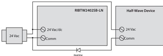
^^ Option 2: Add diode on 24 Vac power (Comm) interconnection between devices. Band on diode faces towards RIB(s).
