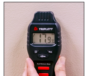
Moisture Meter (pin/pinless)
