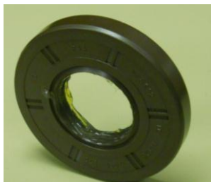
Picture #2 Grease Seal lip before installation.
