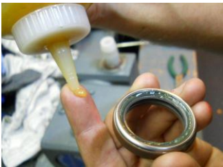
Picture #1 Grease and fill seal cavity by the garter spring
