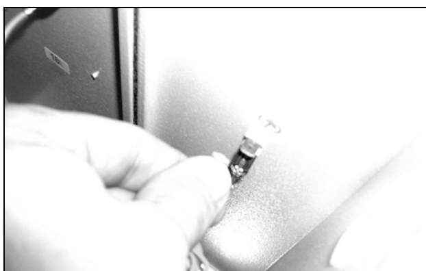
Fig. 73: Disconnect the fan earthing cable (2)
