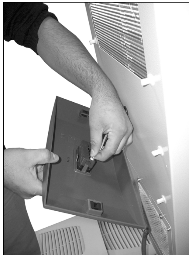
Fig. 42: Disconnect the connector from the display (1)
