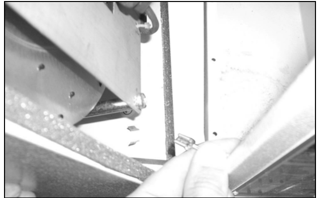
Fig. 54: Loosen the earthing cable between the cover and the chassis (2)
