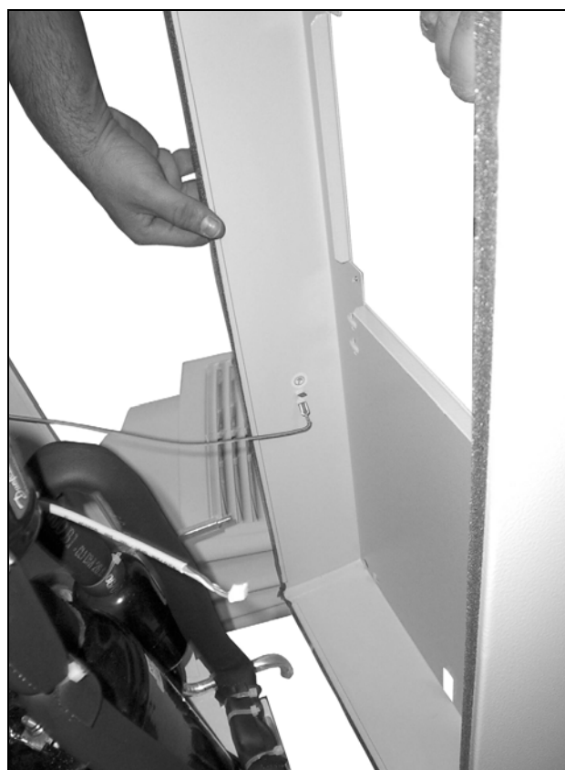
Fig. 76: Disconnect the earthing cable (1)
