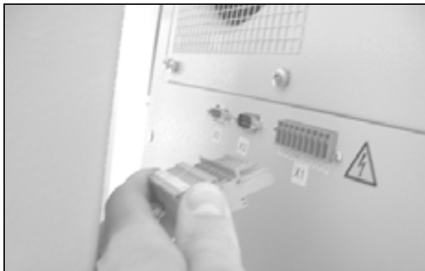
Fig. 38: Disconnect the power cord
