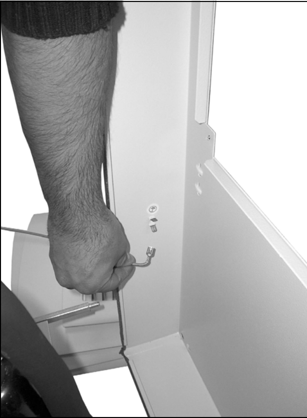
Fig. 77: Disconnect the earthing cable (2)
