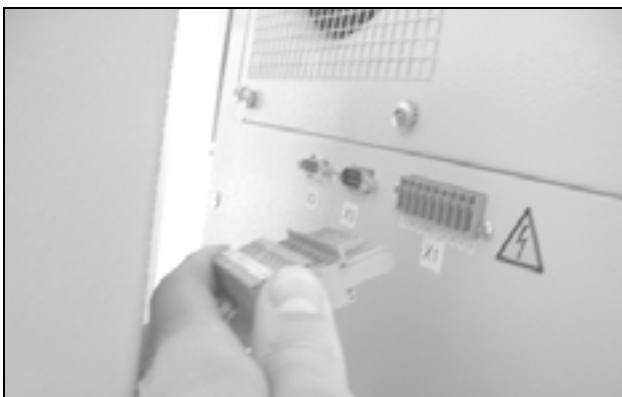
Fig. 57: Disconnect the power cord
