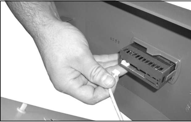
Fig. 64: Disconnect the display cable
