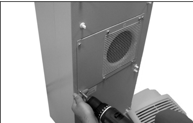
Fig. 67: Loosen the four screws of the external circuit fan
