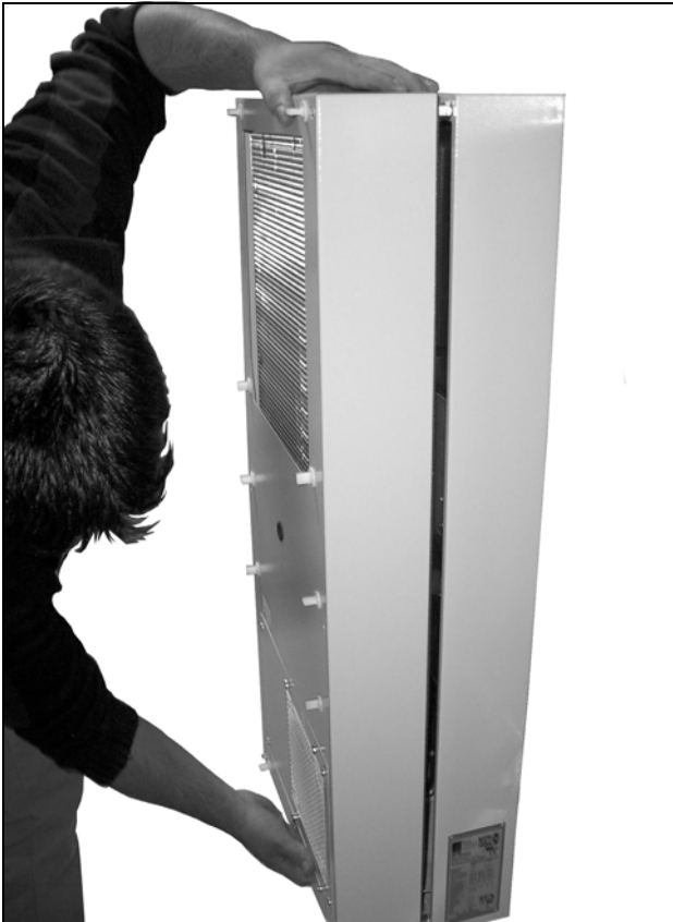
Fig. 51: Remove the cover (1)
