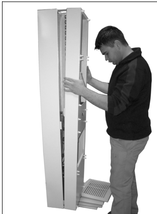
Fig. 75: Remove the cover
