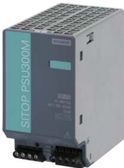
SITOP PSU300M 48V/10A STABILIZED POWER SUPPLY INPUT: 400-500 V 3 AC OUTPUT: 48 V/10 A DC
