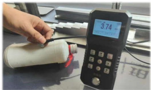
Measure ceramic wall thickness
