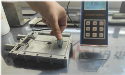
Measure thickness of hollow thin-walled structures
