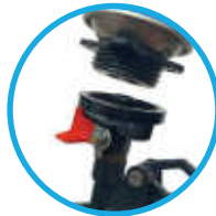
Twist the can lid tightly onto the gun connector to attach it securely.
