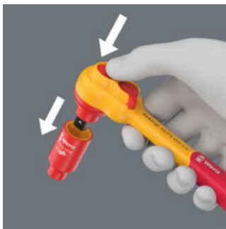
The ball lock ensures sockets and accessories fit securely, providing increased safety during operation. A short press on the release button allows the tool to be changed quickly.
